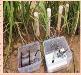
change on the soil moisture sensor output. This ruggedness enabled the low-cost sensors to be used for monitoring soil moisture content at 20 cm or more depth. The low-cost sensor system was conceptualized, developed, and evaluated under the NAHEP CAAST-SNRM project that was compared with the commercially available sensors and found to be at par in moisture prediction. Therefore, the low-cost sensor system can be used in farmer's fields for the precise application of water.
