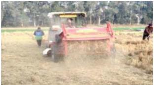
A straw combine was modified for harvesting and chopping of paddy straw. Harvesting and straw bruising units were modified. The machine was evaluated for chopping paddy straw in a combine harvested paddy field. About 85% of paddy straw was having chopping size of less than 12.5 cm. The machine will be evaluated in the coming season for wheat straw.
