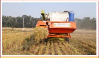
Baling system has been mounted with combine harvester. A flat belt conveyor system was developed and selected for conveying the loose paddy residue falling from the straw walker to the feeder assembly of the baling attachment. The data analysis to check the performance of the combine harvester with the baler attachment is in progress.
