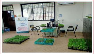
An automated Grafting Robot implements clipping, moving, positioning, cutting, binding and wrapping rootstock and scion saplings
